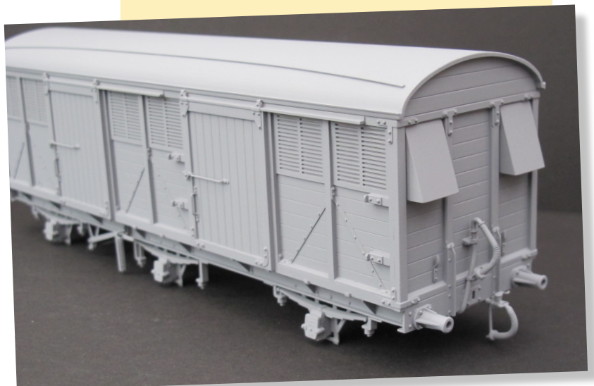
ABOVE and BELOW: Two further views of the LMS D1873 Fish Van under construction. The end ventilator hoods were built up from sheet styrene on the Slater's end mouldings
