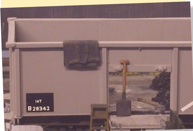
Empty coal sacks wrapped over wagon sides or on lorries are easily modelled using metal foil, such as that found on wine bottles, etc. The rope handle is made of fuse wire, and two slivers of styrene.
