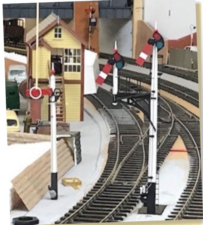
ABOVE: Test fitting the Dapol GW bracket signal - as the servo-mechanism had not been fitted, both arms are 'off'. The Ratio wooden post signal on the left will be replaced by a similar signal with 'cash register' mechanical indicator.
